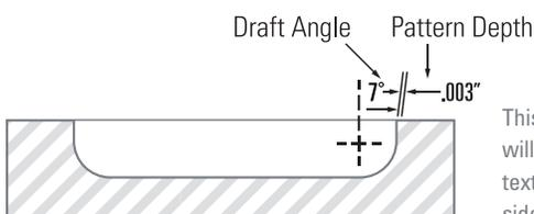
This rule is specific to shrink-away sidewall applications. Areas in the tool that will shrink-on to steel will require 3 times the amount of draft. Lifters, slides, and other tooling components should have their texture draft evaluation based from their angle of action in the tool. Shut-off conditions on textured sidewalls will require additional draft or special work to release parts cleanly.
